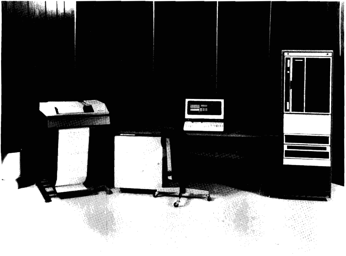
The HP 2026 system may be expanded with peripherals to meet specific customer environments. This configuration would be typical of a central 2026 location and/or an application development system.
